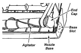
Press firmly, checking to see that each end is completely inserted.
